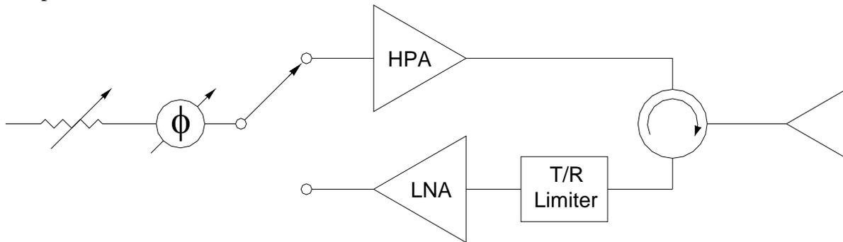
Figure 3-1: Block diagram of a typical solid state T/R module.
