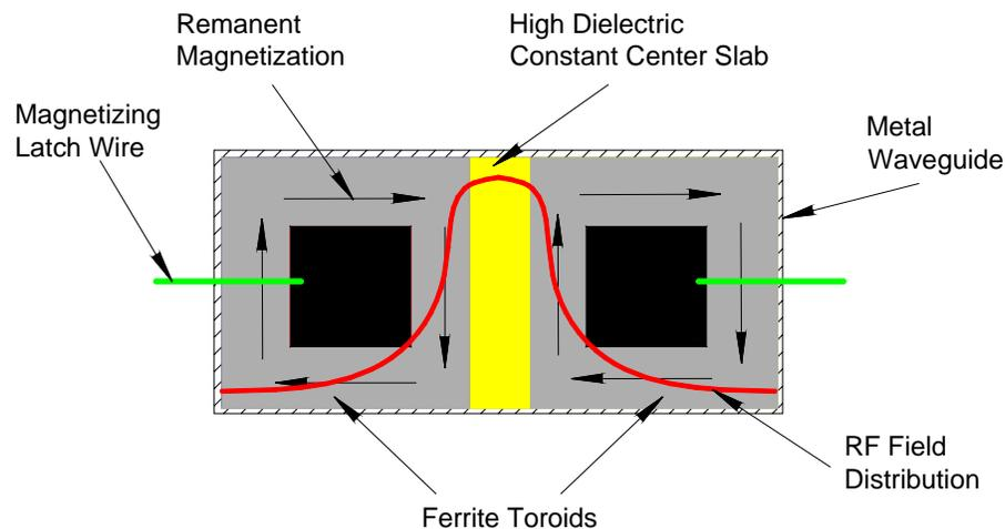
Figure 4-3: Cross section of a dual toroid ferrite phase shifter magnetized in the electrically longest state
