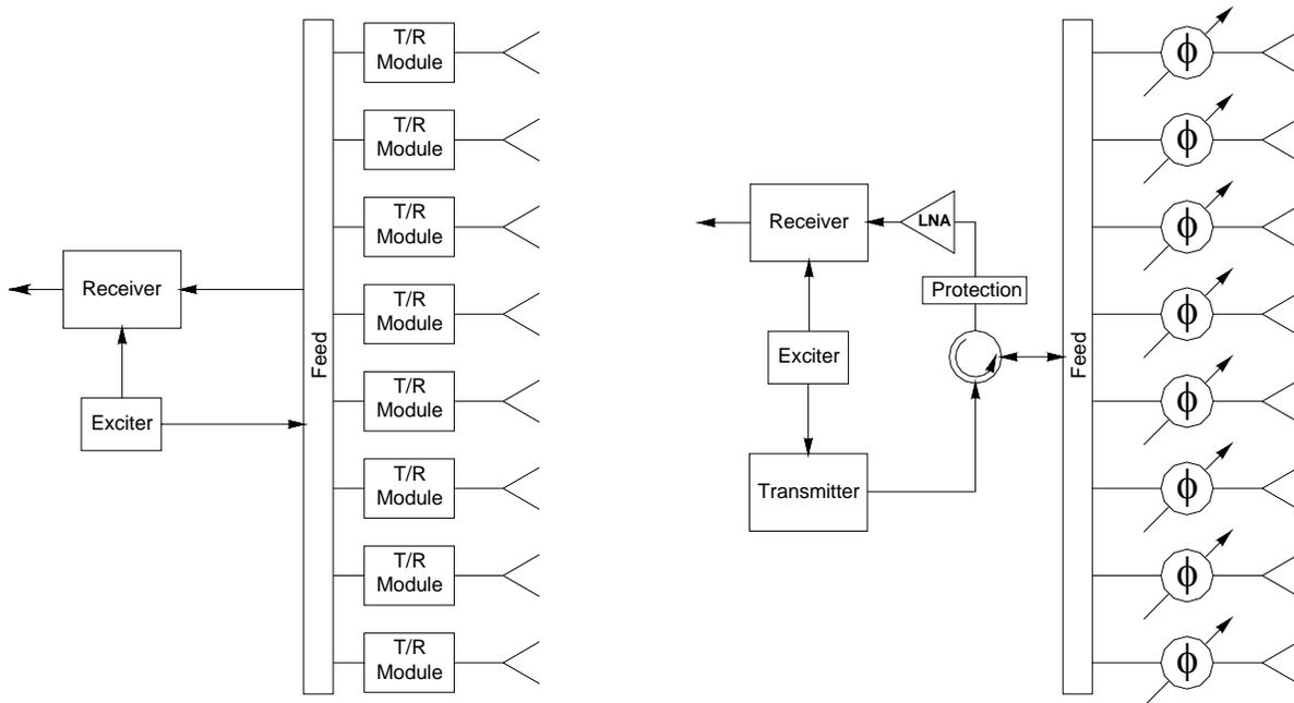
Figure 2-1: Block diagrams of active and passive phased arrays
